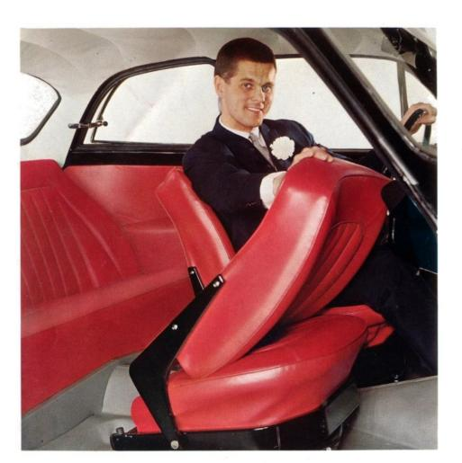
Wide doors with a large opening angle give convenient entry. The hinges and locks are massively dimensioned to give stability and safety. Large map-pockets on the doors. The front seat backrests can be adjusted to three different angles. For reasons of safety they are automatically locked in the front and rear positions. When the backrests are folded down there is plenty of room for comfortable access to the rear seat. The rear side windows can be opened slightly for draught-free ventilation.
